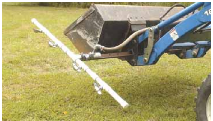
Lehman drives through his orchard, raising and lowering the loader to control width of area to be watered.
