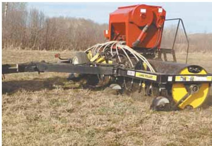
**Heavy-duty blade system mounts in front of Ag Shield land roller to level lumpy pastures or hay fields. Rig can also be fitted with an air seeder for interseeding pastures.**
