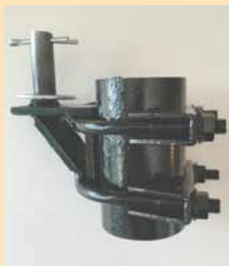
**Clamp-on gate hinge attaches with 2 muffler clamps to a 2 1/2-in. dia. metal post.**
