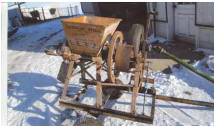
**"Works great to grind small amounts of feed," says Marcus Yoder, who converted an old burr mill to pto power, using a rubber tire to friction-drive the belt pulley.**
