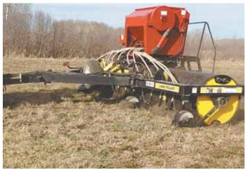
Heavy-duty blade system mounts in front of Ag Shield land roller to level lumpy pas-tures or hay fields. Rig can also be fitted with an air seeder for interseeding pastures.
