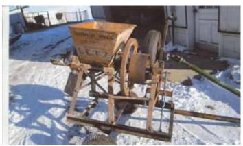
"Works great to grind small amounts of feed," says Marcus Yoder, who converted an old burr mill to pto power, using a rubber tire to friction-drive the belt pulley.
