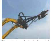
Telescoping boom hydraulically extends Precision Tele-Clipper head from 7 ft. 3 in. to 10 ft. 3 in.
