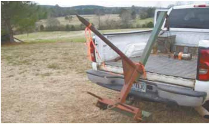
Charles Mitchell doesn't need hydraulic power to pick up round bales with his pickup. Instead, he uses a 1,700-lb. Warn winch to raise and lower the spear.
