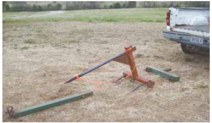
Photo shows the main components of bale spear, which mounts to receiver hitch.
