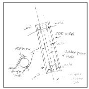
Steering shaft was lengthened by cutting through it and welding in new material with a short length of angle iron behind it.
