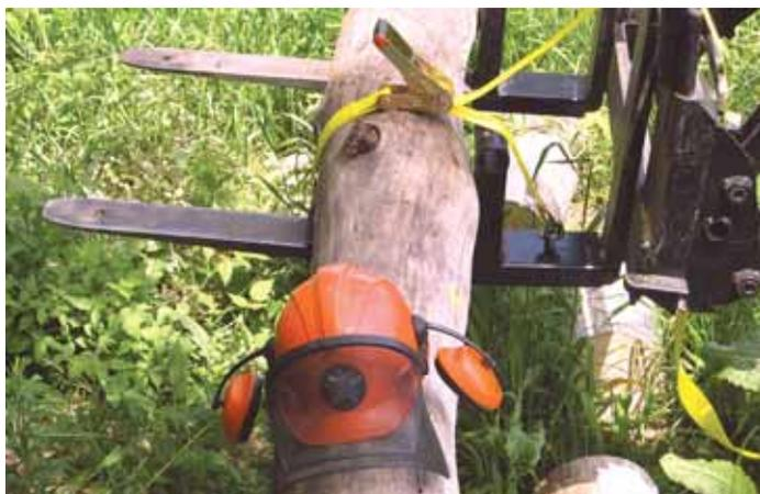
**Tie-down bracket lets Momper saw log while it’s laying on loader forks, so he can stand up straight while sawing.**
