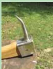
**Pickaroon firewood gripper lets you pick up firewood without bending over. An axehad version is also available.**
