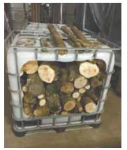
Caddy can be filled with firewood and then moved around with a forklift.
