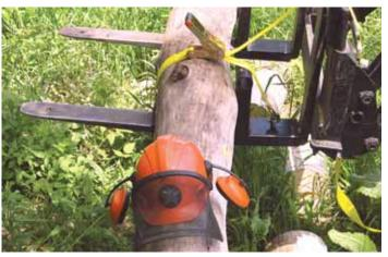
Tie-down bracket lets Momper saw log while it's laying on loader forks, so he can stand up straight while sawing.
