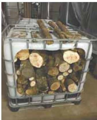
**Caddy can be filled with firewood and then moved around with a forklift.**
