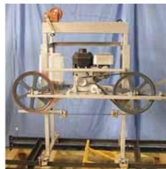
**Saw head rides up and down on 4 metal posts to keep head stable at all times.**
