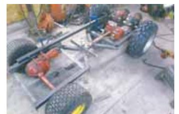
Latimer says building the hydraulic system that operates the drivetrain and mowers was a real challenge.
