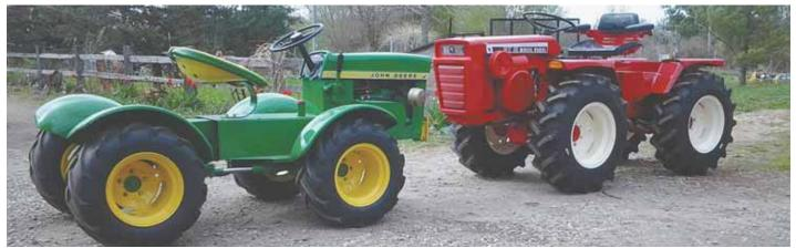
Over the years Bob Rock has produced 12 custom-built articulated garden tractors, including these Deere and Wheel Horse models. All have hydrostatic power and hydraulic steering.
