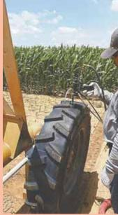
A 3-part polymer is injected into pneumatic tire through a small hole, making tire virtually indestructible.
