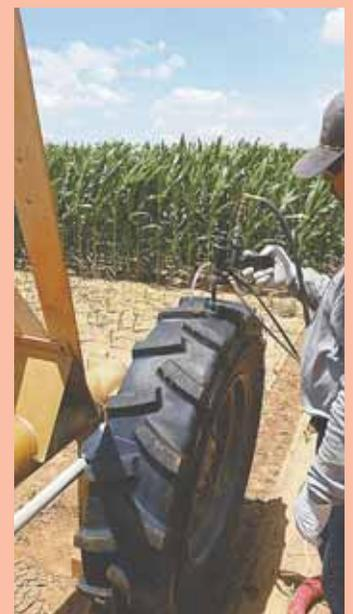
A 3-part polymer is injected into pneumatic tire through a small hole, making tire virtually indestructible.
