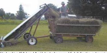
Gies bought an 18-ft. long, 4-ft. wide hay loader, reversed the belt direction, and mounted it in front of a wagon. He mows, rakes and loads 6 acres of hay 3 times every summer.
