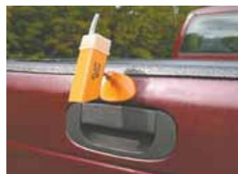
**Ron Adams, Denver, Iowa:** Ron’s pleased with his Swift Hitch portable wireless backup camera ([www.swift hitch.com](http://www.swift hitch.com); ph 617 600-8282). “It’s equipped with a magnetic base and a handheld display with a color 2 1/2-in. LCD screen. I mount the camera on my pickup’s tailgate and aim it at the hitch. It lets me back up to equipment without needing someone to help.”
