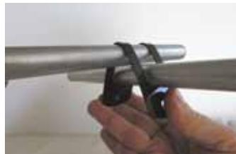
To use the clip you squeeze both ends and slip in pieces of conduit, and then release (left). Spring tension holds conduit tightly in place.
