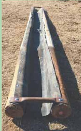
Low-cost cattle feeder was made from telephone poles covered with used conveyor belting.
