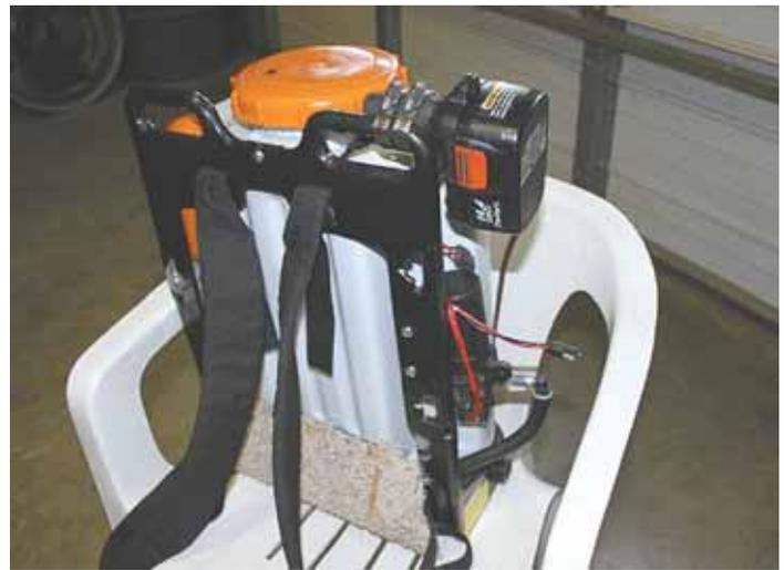
Tired of using the pumping lever on his Stihl manual backpack sprayer, Mike Buss decided to convert it to electric-powered. "The battery runs all day on a full charge," he says.
