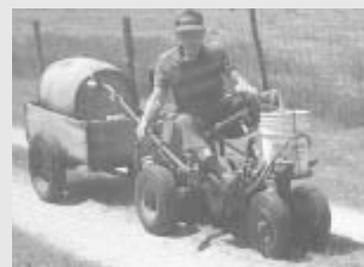
**He turns the machine into a riding tractor by mounting a seat in front of the engine and adding a short frame and narrow spaced front wheels.**
