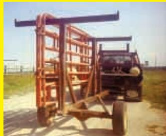
I built a corral panel trailer using the rear axle off an old pickup and some other odds and ends. It's much easier hauling the panels on a trailer than it would be on a truck or with a front-end loader.
