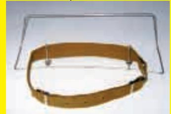
It consists of an L-shaped metal rack, made from 3/16-in. dia. rod, which is attached to a web belt that fits around your waist. The posts simply lay on the rack.
