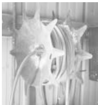
Homemade reel holds 100 ft. of pressure hose.
