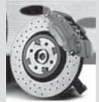
improve braking on drum brakes. He cautions that cross-drilling should not be a do-it-yourself project. "If the rotor is not designed properly, drilling or slotting them can cause brake failure. We've seen cases where pieces of the rotor just break off."
