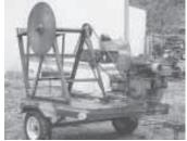
was worn out. I also rigged up a couple of other pulleys and a belt tightener, which I borrowed from the power steering pump on a car.
