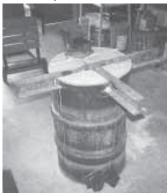
Karey Waldrop, Walterboro, S.C.: "I used a 55-gal. barrel and lengths of old railroad track to make a combination vice table and anvil. The drum was filled with sand to within 8 in. of the top and finished off with rebar and cement. The vise is fastened to bolts that are anchored in the cement.
