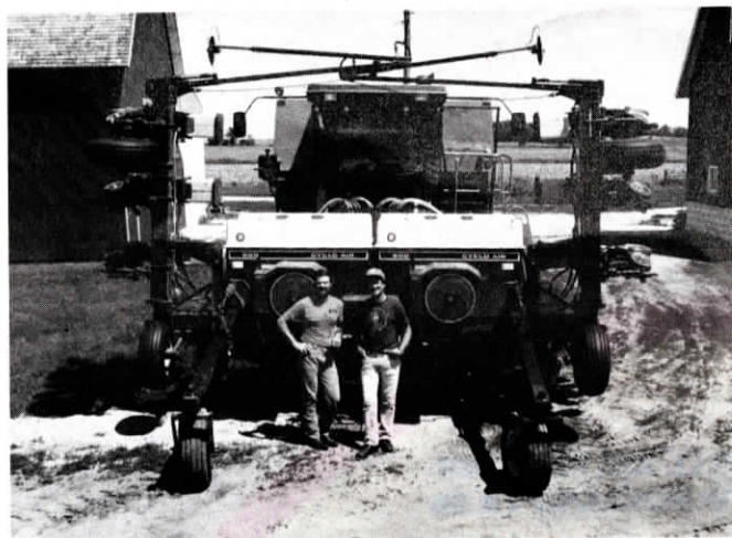
In transport position much of the 12-row planter's weight is supported by the front lift assist wheels, say Dennis Carney and Clayton Black.
