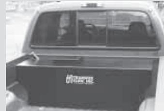
**Chico, Calif. 95973 ph 800 442-0056 or 530 893-5209; website: www.transferflow.com);** This company offers auxiliary fuel tank systems for pickups designed to transfer fuel automatically to the main tank. Its newest offering is a 70-gal. in-bed tank for diesel pickups. It comes pre-assembled and includes the fuel tank, auxiliary fuel pump, fuel lines, wire harness, mounting hardware, and computer module. The computer module will turn
