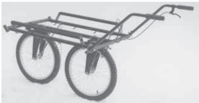
In-line wheels allow Neet Kart to easily climb over logs and other obstacles.
