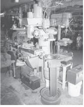
up as much wall space. I keep a portable anvil nearby that I made out of an old wheel rim and a length of railroad track.
