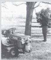
C.F. Marley uses the engine on his garden tractor to belt-drive a generator, which he mounted on front of tractor. It lets him power electric tools such as chain saws and hedge trimmers.
