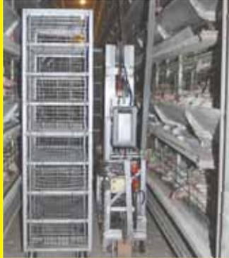
easier and more efficient. It can be operated by either remote control or dedicated controls on the machine. It can lift a full-loaded cart 900 lbs. to a height of 8 ft. Much easier than lifting chickens up and down by hand. To watch a video of it in action go to [www.avianelevator.com](http://www.avianelevator.com). (David Becker, 643 Hereford Road, Elizabethtown, Penn. 17022; ph 717 361-9400; [dcwelding@embarqmail.com](mailto:dcwelding@embarqmail.com)).
