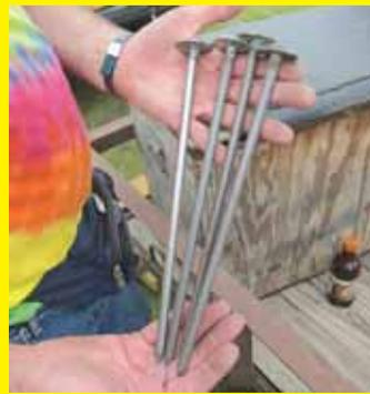
I often attend antique tractor shows and stay overnight in a tent at the show site. I don't like using those long plastic spikes to stake the tent down, because they can easily break when pounded into hard ground. So I went to a local hardware store and bought some cheap 12-in. pole barn nails, then welded 3/8-in. dia. fender washers under the heads to keep the rope from sliding off the nail. (Dave Dam, 111 N. Buena Vista Rd., Eau Claire, Wis. 54703; ph 715 450-2943)
