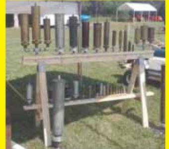
shells ranging from 75 to 105 mm. A pipe with elbows and an air compressor hookup connects the shells together. They are designed to make a triple tone like you find on big ships.
