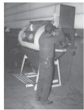
Tank has an air-powered blast gun that's pre-plumbed into a quick-tach air hose.
