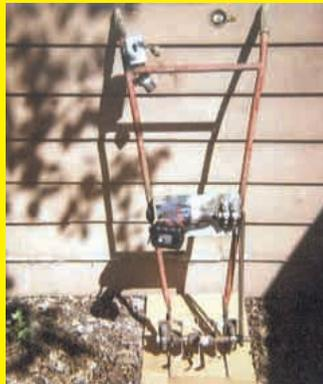
Here's a cultivator I made for tilling in between rows of vegetables. I made some tines out of stainless steel and mounted them between the handles off an old mower. The tines are powered by a 1/2 in. cordless drill that chain-drives the tines. Instead of wheels, I put two skids on it. **(Ken Voigt, Wausau, Wis.)**
