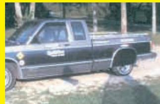
I wanted to add wheel skirts on back of my 1991 Chevy S-10 pickup but couldn't find any, so I made my own out of aluminum sheeting. The sheeting was left over after someone added aluminum trim around the windows of my house. I cut it to shape and used self-threading screws to attach it to the chrome trim around the pickup's rear wheels. The aluminum is painted purple and green, the same color as the pickup. **(Doug Brown, Columbia, Tenn.)**
