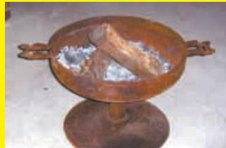
I took an old 65-gal. propane tank, filled it with water, and then carefully cut the end caps off. The base is a 20-in. smooth disk blade with an 8-in. piece of 2 5/16-in. dia. pipe. The handles are sickle guards off a 750 MF Combine 16 ft. header.
