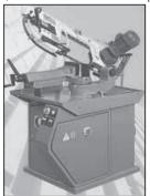
with this one. It's powered by a 2 hp electric motor and has a recirculating fluid cooling system that allows me to cut through 4-in. solid metal in only 2 1/2 to 3 minutes. It has a 37-in. working height and can cut at up to a 60 degree angle, which makes it a pleasure to operate."
