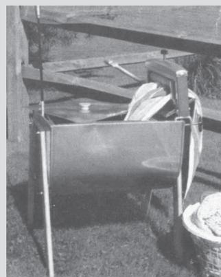
The James Hand Washer can be fitted with a wringer roller at one end.
