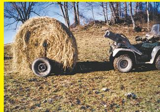
I haul 4 by 5-ft. 800-lb. round bales and unroll them on the ground with a 450 Honda. I just lower the arms down on either side of a bale and stick the spikes into the center of the bale. Then I use a
