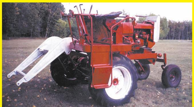
I don't know what to call this machine but I made it from an old combine. It's very maneuverable and easy to operate and can do the work of a tractor. I made it from an old combine, removing all the threshing components and leaving just the frame. I remounted the engine lengthwise, added an angle gear drive
