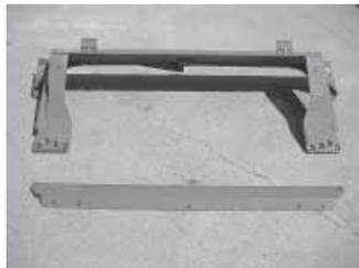
Upgraded feeder house tilt frame for Deere Contour Master combines.
