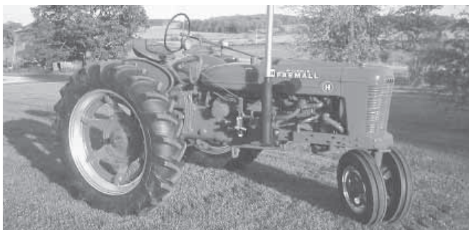
Lloyd Statz repowered his Farmall H with a Mercedes Benz 2.2-liter, 4-cyl. diesel engine. "It runs smooth and looks like it belongs in there," he says.
