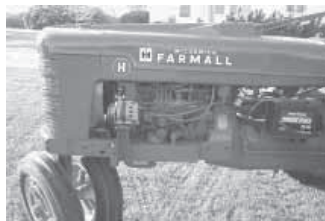
A pulley off another IH tractor is used to belt-drive tractor's original fan.
