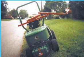
Weight Arm Balances Mower On Slopes
