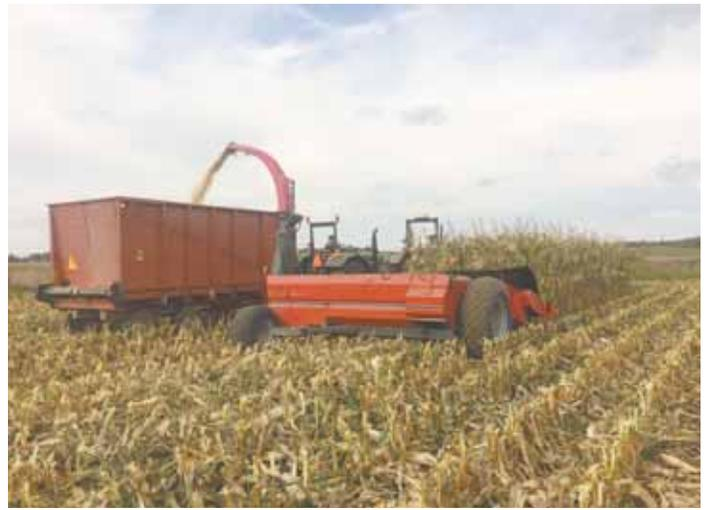
Crop enters from the cornhead through the feederhouse to a feeding auger, which pushes it into the cutterhead. Material then moves to an impeller blower off a Dion forage harvester.
