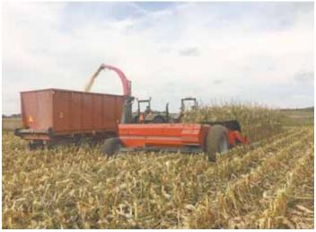
Crop enters from the cornhead through the feederhouse to a feeding auger, which pushes it into the cutterhead. Material then moves to an impeller blower off a Dion forage harvester.
