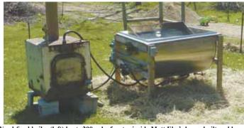
Wood-fired boiler (left) heats 200 gal. of water inside Matt Eby's home-built scalder.
