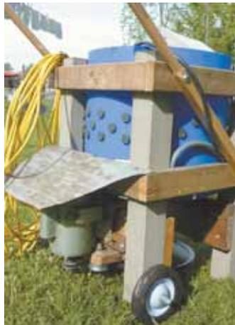
He built this plucker using a cut-down, food grade plastic barrel set in a wooden frame.
