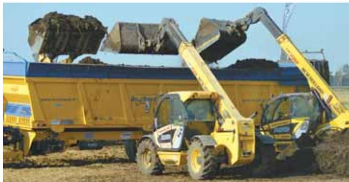
This 7-ft. wide, 40-ft. long spreader box has a total heaped capacity of 55 tons of solid manure. It recently set a world record by spreading 4,648 tons of manure in 24 hrs.
