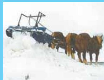
Once blade is filled with snow, Fisher releases a chain which causes panel to tip forward and glide over the gathered snow.
