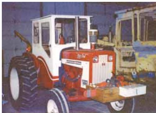
Douglas Strouse built this cab for his IH 504 tractor. It’s designed to be lifted off the tractor using a shop crane.
