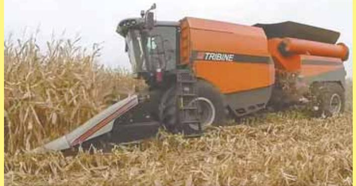
Revolutionary articulated Tribine combine recently went into production. It has a trailing grain tank fed by a 12-in. auger. Chaff and straw blows out in front of tank.
