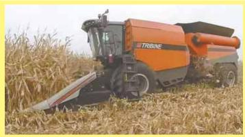
Revolutionary articulated Tribune combine recently went into production. It has a trailing grain tank fed by a 12-in. auger. Chaff and straw blows out in front of tank.
