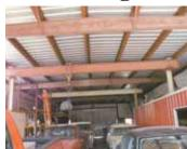
Overhead shop hoist moves back and forth on a 24-ft. long I-beam supported at each end by a vertical steel beam.
