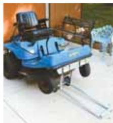
**Egleston pushes dolly forward to engage lift fingers into lift rod, and then pulls the lift handle forward and down to the ground.**
