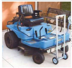
Dolly lift has a pair of 9-in. long horizontal lift fingers on front fitted with 2-piece metal brackets, which form a cradle for a metal "lift rod" bolted on under mower.
