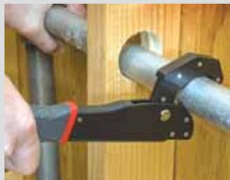
The self-adjusting head instantly grabs and releases pipes. You position the wrench around the material, then press the head forward or pull up on the jaw to release and re-engage.
