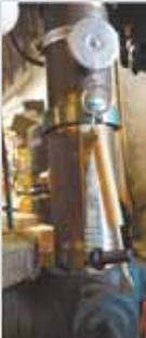
"I took a metal key holder with retractable cable and fastened it with a hose clamp to the drill press post. Then I attached the chuck key to a wooden dowel and hooked it to the retractable cable. Problem solved."
