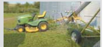
**Rex Gogerty, Hubbard, Iowa:** "We used a jack to raise the rear end on our Deere lawn tractor in order to keep the pto level with the pto on our grain auger. We also raised the tractor's front end so we can keep the engine oil level, making the engine less likely to overheat."
