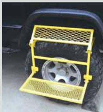
and then fold the steps down. A pair of wide tabs welded onto the back side of the frame come in contact with the tire to keep the frame from damaging the sidewall. The steps are made from powder-coated expanded metal and designed to hold up to 500 lbs. They're available in bright red or safety yellow for high visibility.
