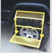
and then fold the steps down. A pair of wide tabs welded onto the back side of the frame come in contact with the tire to keep the frame from damaging the sidewall. The steps are made from powder-coated expanded metal and designed to hold up to 500 lbs. They're available in bright red or safety yellow for
