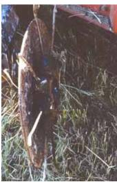
Fritz Dillon removed the worn-out rubber lining on the gathering wheels of his round baler and welded teeth off a junked rake onto both sides of the wheels.
