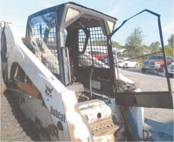
Cab enclosure consists of clear vinyl windows on all sides with a hinged door. It fits onto the existing cab frame with Velcro and bungle cords.
