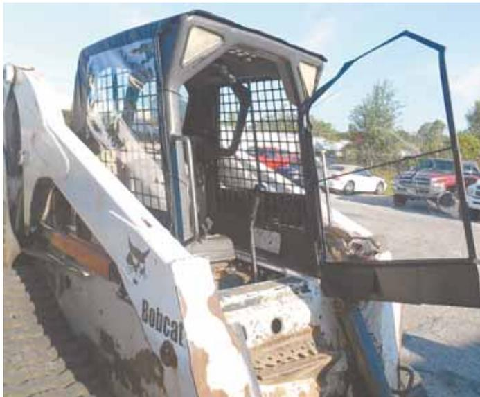
Cab enclosure consists of clear vinyl windows on all sides with a hinged door. It fits onto the existing cab frame with Velcro and bungee cords.
