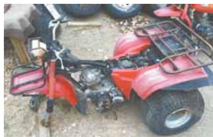
He stripped an ATC 200E 3-wheeler down to the frame and removed the engine, then fabricated a swing-arm mount.
